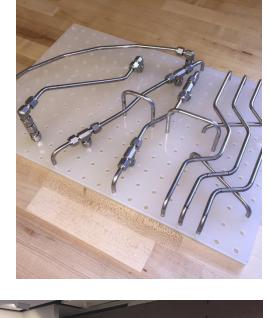
Installation and Tube **Bending Safety Essentials** class includes a two-hour introductory segment that demonstrates how to assemble a tube fitting. Balance of day is then devoted to student mastering the use of a hand tube bender to make bends of 45°, 90°, 180°, and offsets. Time is also spent learning how to
