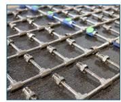
**Orbital Welding** Achieve quality welds on stainless steel tubing or other alloys upon request. Our welders are certified in ASME Section IX standards.
