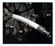
Hose Assemblies Choose from a vast selection of hose products, then let us cut them to your specified length and fabricate custom end connection configurations.
