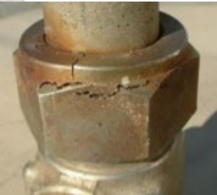
10.1% nickel content 316 stainless steel nut from another manufacturer shows cracking after installation in a corrosive environment.
