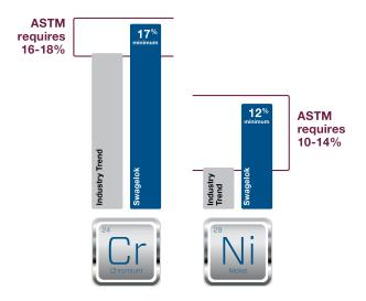
Chromium and nickel are critical for corrosion resistance and ductility in stainless steel. Swagelok has maintained chromium content in its fittings at a minimum of 17% and nickel at a minimum of 12% for many years.
