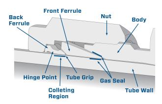
Swagelok tube fittings have a grip-type design that uses a unique "hinging and colleting" action to achieve optimal performance in three key areas:
