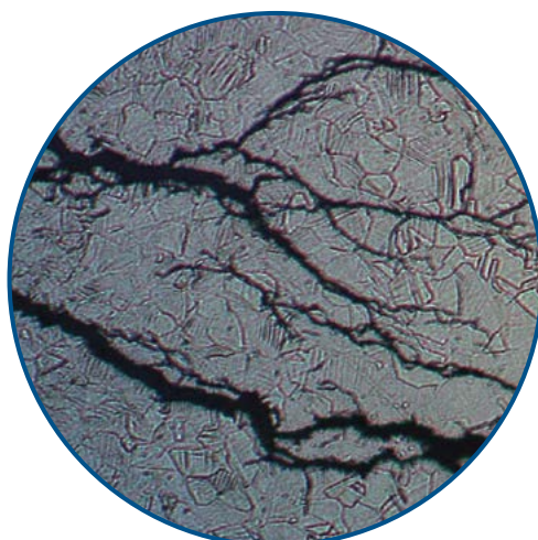
Stress Corrosion Cracking
