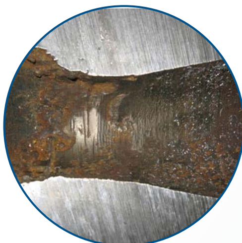
Sour Gas or Sulfide Stress Cracking
