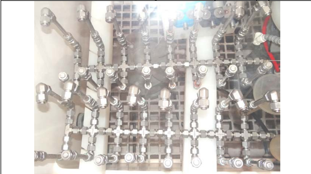
Assembled and Pressurized Tube Fittings Installed in Cyclic Salt Spray Chamber
