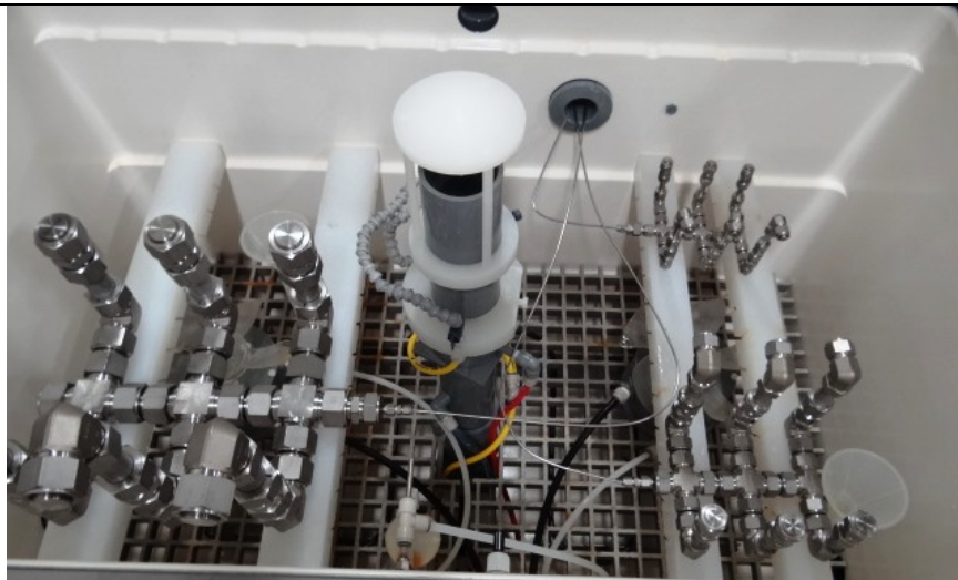
Assembled and Pressurized Tube Fittings Installed in Cyclic Salt Spray Chamber
