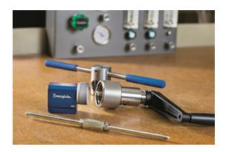
The manual coning and threading tool is designed to cone and thread 1/4, 3/8, and 9/16 inch Swagelok® IPT series tube in order to make tube nipples. The tools are designed with interchangeable coning blades, bushings and threading dies.
