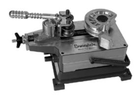
Swagelok® Bench Top Tube Bender has a rugged, lightweight aluminum construction and is ready to bend 1/4 to 1 1/4 in. outside diameter (0.028 to 0.120 in. wall thickness) and 6 to 30 mm outside diameter (0.8 to 3.0 mm wall thickness) tubing range.
