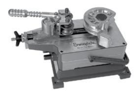
Swagelok Bench Top Tube Bender has a rugged, lightweight aluminum construction and is ready to bend 1/4 to 1 1/4 in. outside diameter (0.028 to 0.120 in. wall thickness) and 6 to 30 mm outside diameter (0.8 to 3.0 mm wall thickness) tubing range.
