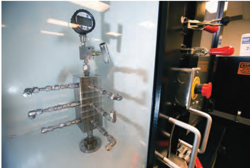
Figure 7-9 Hydraulic impulse test.
