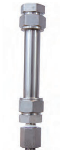
Figure 7-11 Tubing yield before burst.
