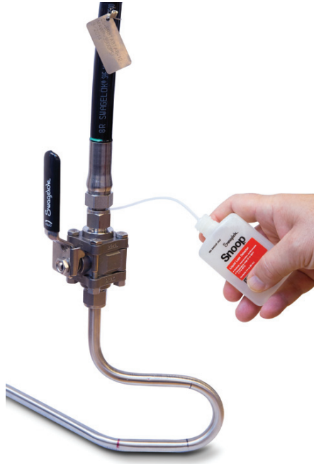
Figure 7-3 Snoop leak test.
