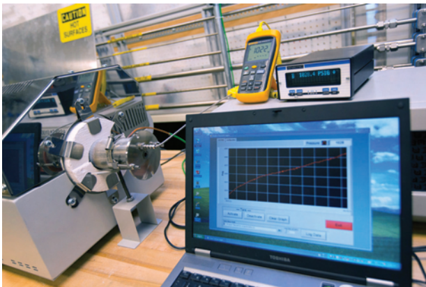
Figure 7-13 1000 psig (68 bar) gas test at 1000°F (538°C).
