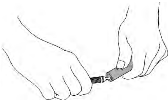
Figure 3-51 ID deburring with a Swagelok deburring tool.
