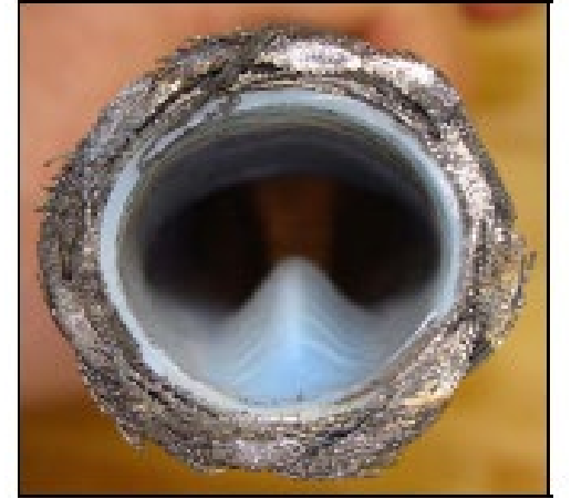
Cross section of a kinked hose
