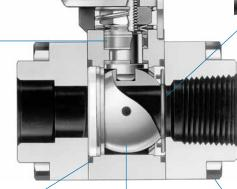
Compensating seat design live loads the seat to compensate for wear and changes in temperature or pressure during normal conditions and reduces distortion of seats from pressure surges
