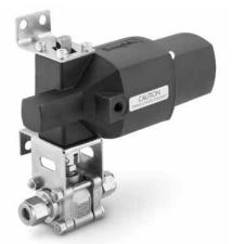
Swagelok rack and pinion pneumatic actuators are compact, lightweight, easily mountable, and can be operated with standard shop air. They are available in spring-return and doubleacting modes. On-off (2-way) valves require 90° actuation; switching (3-way) valves require 180° actuation.
