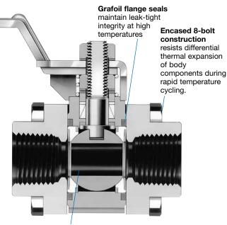
The Steam 60 Series Ball Valves have a smaller orifice than the standard valves for improved seat sealing performance after thermal cycling. The maximum  $C_{\nu}$  of the Steam 60 Series valves is shown in the table below. User should compare this to the  $C_{v}$  in the end connection tables above, to see if the maximum  $C_{\nu}$  is reduced.
