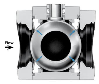
Under high pressure, the ball is forced downstream, flexing the downstream seat and creating a seal. The upstream seat also flexes with the ball movement and maintains a seal.
