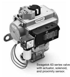
These Swagelok rack and pinion pneumatic actuators are ISO 5211 compliant and are suitable for general applications. They are available in spring-return and double-acting modes. On-off (2-way) valves require 90° actuation; switching (3-way) valves require 180° actuation (90° actuation for valves with L flow pattern).
