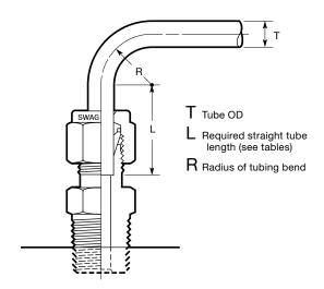
Tubing properly selected and handled, combined with properly installed Swagelok tube fittings, will give you a leaktight system and provide reliable service in a wide variety of applications.
