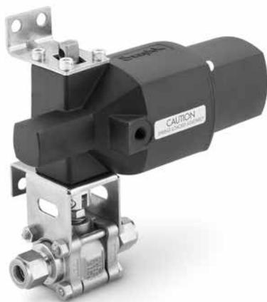
Swagelok rack and pinion pneumatic actuators are compact, lightweight, easily mountable, and can be operated with standard shop air. They are available in spring-return and double-acting modes. On-off (2-way) valves require 90° actuation; switching (3-way) valves require 180° actuation.
