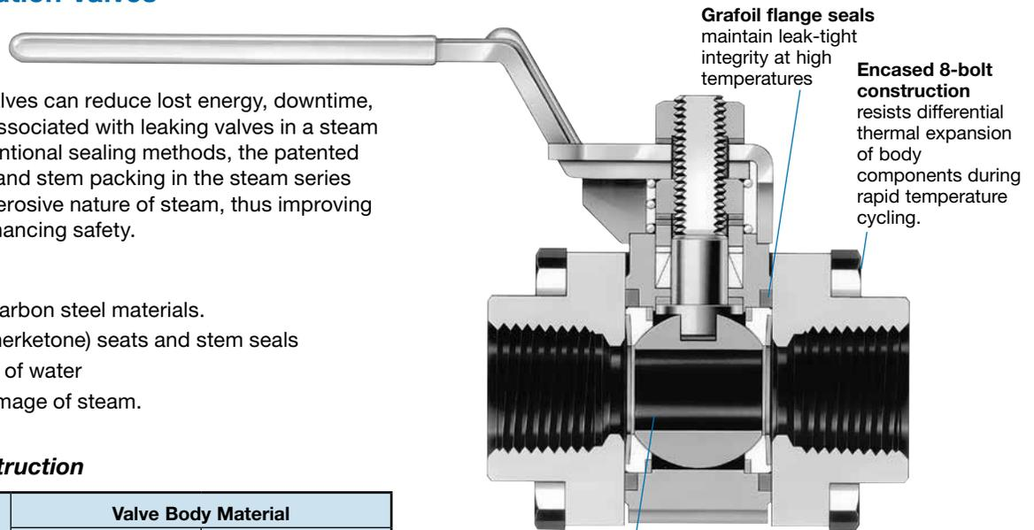
The Steam 60 Series Ball Valves have a smaller orifice than the standard valves for improved seat sealing performance after thermal cycling. The maximum  $C_v$  of the Steam 60 Series valves is shown in the table below. User should compare this to the  $C_v$  in the end connection tables above, to see if the maximum  $C_v$  is reduced.
