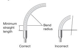
Hose rupture or leakage may result from bending too close to the hose/fitting connection.
