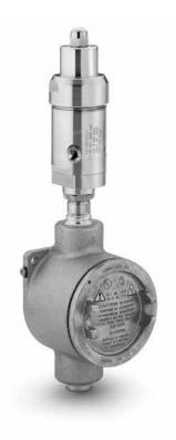
The KEV series is an electrically heated vaporizing regulator with a low internal volume. It can be used to vaporize liquid samples or to preheat gas samples to prevent them from condensing. It features a heating element that is in direct contact with the process fluid for maximum thermal efficiency and is removable for easy cleaning. The KEV regulator has an integral temperature controller and is rated for use in hazardous areas, as identified below.
