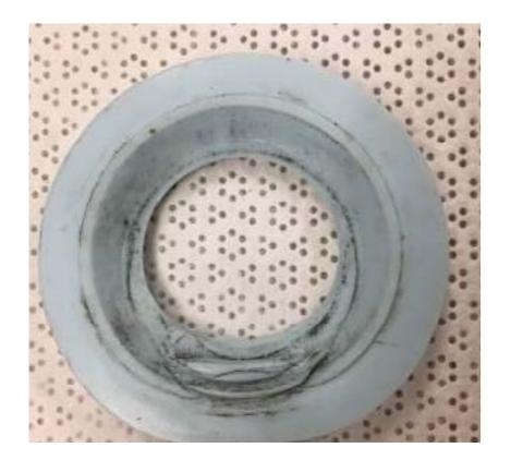
Example of the effects of cold flow on PTFE that can result from operating a valve in the partially open position for a prolonged period of time, or if the valves are operated under pressure in the partially open position.
