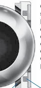
Compensating seat design live loads the seat to compensate for wear and changes in temperature or pressure during normal conditions and reduces distortion of seats from pressure surges
