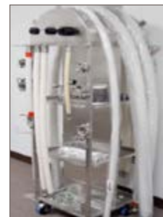
Figure 3. Proper hose storage requires hanging hoses and ensuring they are not bent more than their published bend radius.
