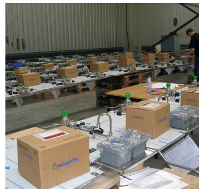
Swagelok Nederland provided kits of individually packaged components, packaged according to assembly instructions per sampling system.
