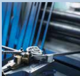
Tube Bending and Cutting
