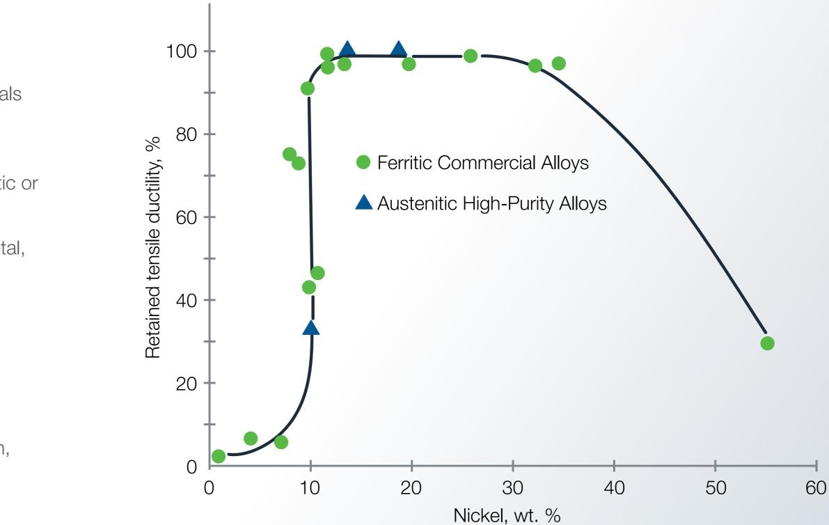
Ferritic alloys with very low nickel content become significantly embrittled, while austenitic alloys with nickel content between 10% and 30% show relatively little embrittlement.
