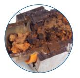
**Galvanic Corrosion** Can occur when two dissimilar materials are in intimate contact with each other and an electrolyte is present
