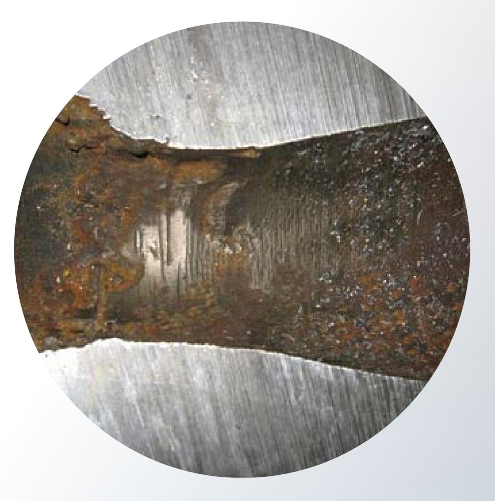
Reprinted from Science Direct, Volume 1, Issue 3, S.M.R. Ziaei, A.H. Kokabi, M. Nasr-Esehani, Sulfide Stress Corrosion Cracking and Hydrogen Induced Cracking of A216-WCC Wellhead Flow Control Valve Body case study, Pages 223-224, July 2013 with permission from Elsevier.
