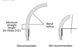
Hose rupture or leakage may result from bending too close to the hose/fitting connection.
