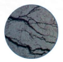
Stress corrosion cracking (SCC) is dangerous because it can destroy a component at stress levels below the yield strength of an alloy. In the presence of chloride ions, austenitic stainless steels are susceptible to SCC. The ions interact with the material at the tip of a crack where tensile stresses are highest, making it easier for the crack to grow. While in progress, SCC can be difficult to detect, and final failure can occur suddenly.
