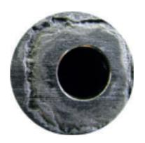
In a typical fluid system, crevices exist between tubing and tube supports or tube clamps, between adjacent tubing runs, and underneath dirt and deposits that may have accumulated on surfaces. Crevices are virtually impossible to avoid in tubing installations, and tight crevices pose the greatest danger for corrosion to occur.
