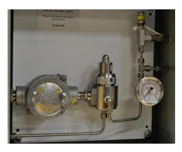
This electrically heated vaporizing regulator is a critical part of this sample conditioning panel. Being coupled with an outlet gauge and relief valve, this panel provides protection for the expensive instrument it feeds.
