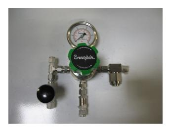
Safe delivery of gas bottle pressure is achieved with this regulator. A filter upstream protects the diaphragm and ensures a long service life. The attached relief valve guards against over pressurizing the line when adjustments are made to the regulator knob. The downstream block valves allow for depressurizing and purging of the delivery system from the source through the regulator.
