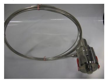
This high sensitivity regulator is used in a toxic service. The regulator has a captured vent and the customer was very interested in having product vented to a safe location. Having the fitting assembled by Swagelok certified installers to ensure no leakage, along with no extra potential leak paths from a 50 foot coil of tubing was important for a safe installation. Having this packaged as one piece ensured that all parts were in place for safest installation.
