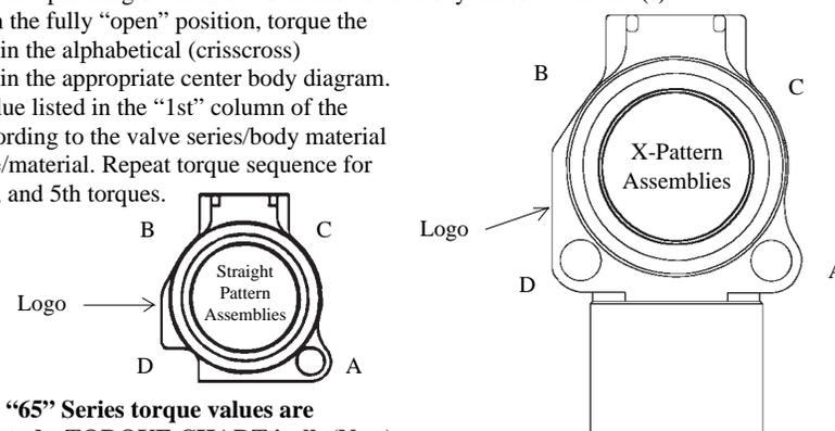
**NOTE: "62" through "65" Series torque values are the same for bolts or studs. TORQUE CHART in·lb (N·m)**
