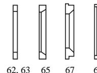
**NOTE:** "65", "67", and "68" Series support rings are installed with the chamfered side toward the ball.
