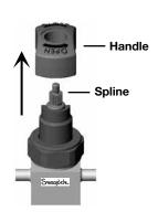
4. Place the new directional handle on the spline, aligning the OPEN label over the front of the valve body. Handle will be perpendicular to the ports.
