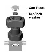
3. Turn handle to the CLOSED position, then lift up on the handle and remove from valve.
