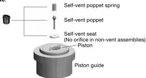
8. Push the **piston** out of the **piston guide**.
