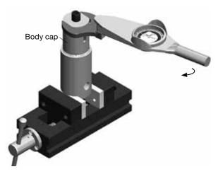
24. Place the **handle** and the **handle retainer** on the **body cap**.
