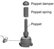
15. Invert the **body** and **seat assembly** and thread the seat assembly into the body.
