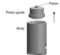
6. Lightly grip the **piston guide** in the vise and loosen the self-vent seat retainer from the piston guide using the **piston assembly bar** and **vent retainer tool**. The piston assembly bar must be held still.
