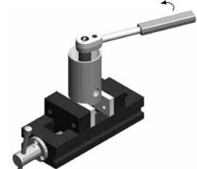
11. Invert the body and remove the **seat retainer**. Then remove the **poppet damper**, the **poppet spring**, **poppet** and the **seat** from the **seat retainer**.
