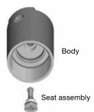
Tighten the seat assembly to: for non-metallic seat: 13 ft·lb (17.5 N·m, 1.8 m·kg) for metallic seat: 26 ft·lb (35.0 N·m, 3.7 m·kg)
