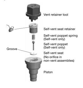
20. Insert the piston into the piston guide. Lightly grip the piston guide in the vise and tighten the self-vent seat retainer to 7 ft·lb (10 N·m) using the **piston assembly bar** and **vent retainer tool**.
