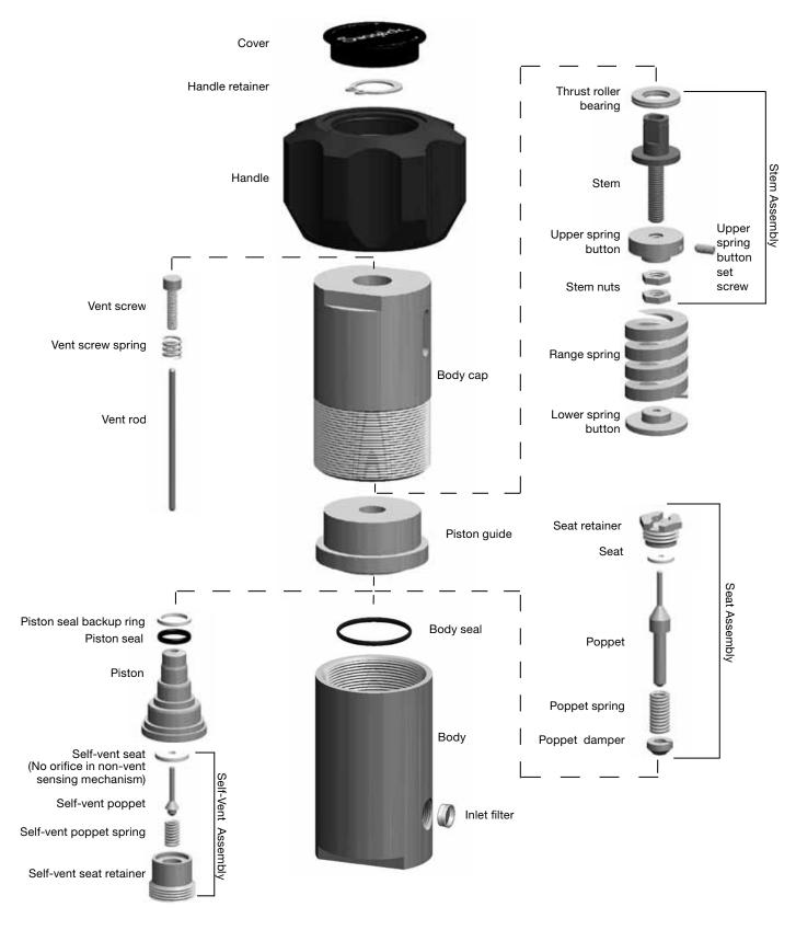
Note: Regulators with no self-vent option do not contain a vent screw, vent screw spring, vent rod, self-vent poppet, and self-vent poppet spring.
