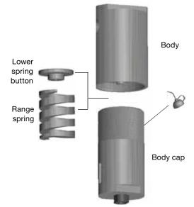
23. Tighten the **body cap** to 129 ft·lb (175 N·m, 17.9 m·kg).
