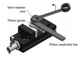
7. For regulators with a self vent, remove the **self-vent poppet spring** and the **self-vent poppet.** For all regulators, remove the **self-vent seat** from the **piston guide**.
