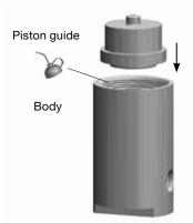
22. Place the **range spring** and the **lower spring button** into the **body cap**. Thread the body cap finger-tight into the **body** in the inverted position.
