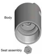
14. Tighten the seat assembly to 13 ft·lb (17.5 N·m).
