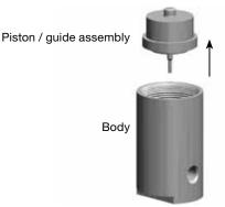
Lightly grip the piston guide in the vise and loosen the poppet retainer from the piston / guide assembly using the piston assembly bar and the vent retainer assembly nut. The piston assembly bar has to be held still.
