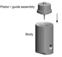
Place the range spring and the lower spring button into the body cap. Then thread the cap assembly into the body in the inverted position.
