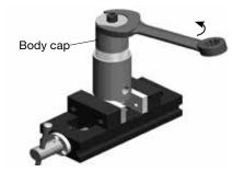
Remove the cap assembly from the body.
