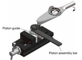
Insert the piston / guide assembly into the body. Lightly press down on the piston guide until it is fully seated.
