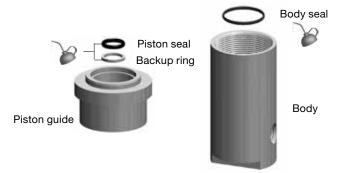
Insert the **piston assembly** into the **piston guide**. Lightly grip the piston guide in a vise and tighten the poppet retainer to 7 ft·lb (10 N·m).
