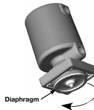
5. Thread the **new diaphragm** into the actuator assembly until it is finger-tight.
