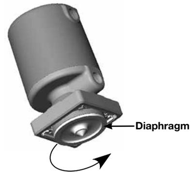
4. Thread the **new diaphragm** into the actuator assembly by holding the diaphragm on the outer edge and rotating the diaphragm *clockwise*.
