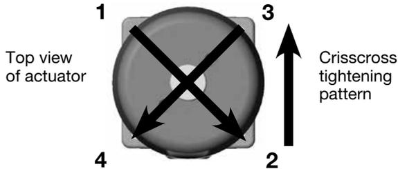
⚠ **Plastic Actuators ONLY: After the cap screws have been torqued, no gap should be visible between the actuator housing and the body. If there is a gap, tighten the cap screws.**
