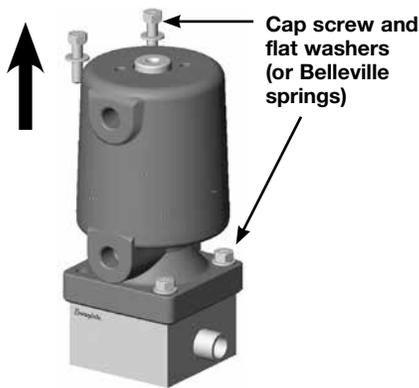
4. Remove the **actuator assembly** from the valve body.
