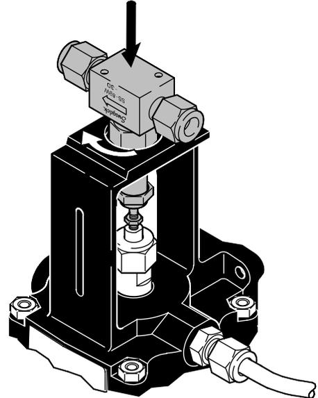
2. Lower the valve through the actuator flange and the flange nut.
