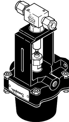
This document describes how to replace a 3 series actuator with a 5 series actuator. These instructions apply to double-acting (D), normally open (O), and normally closed (C) models. The illustrations above show the assemblies before and after replacement.
