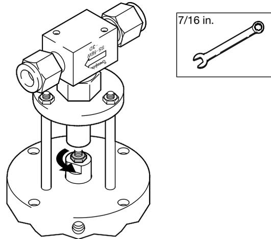
7. Unscrew the valve from the piston rod and remove the valve from the actuator.
