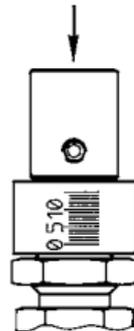
**STEP 4** Loosen **Stem Extension Screw** and slide **Stem Extension** down against **Barrel** maintaining stem position. Retighten **Stem Extension Screw**. A positive handle stop is now set.
