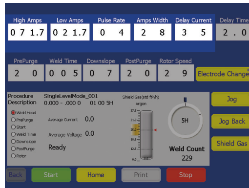
Fig. 63—Single Level Current-Control Group
