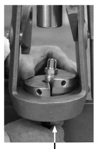
12. Remove one **die** from the **housing** while holding the **swaged assembly**. Remove the swaged assembly through the bottom of the housing.
