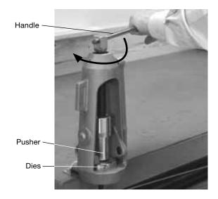
9. Rotate the **handle** counterclockwise until the **pusher** has reached the top of the **housing**.
