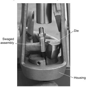
Inspect the first swaged assembly to ensure it is within tolerance prior to swaging additional end connections of the same hose size and type.
