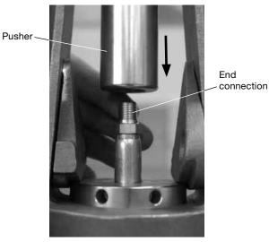
8. Continue to turn the **handle** clockwise until the **pusher** makes contact with the **dies**. The swaging action is finished when the handle will no longer turn.
