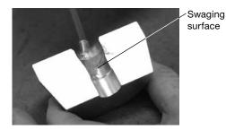
8. Insert one die into the taper at the base of the housing. Do not secure the die clamp at this time.
