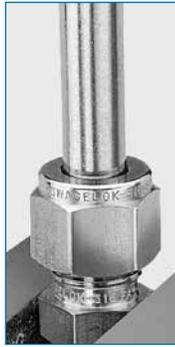
1. Insert cleanly cut, fully deburred tube into the depth marking tool (DMT) until the tube is against the shoulder of the tool. Using a pen or pencil, mark the tube at the top of the DMT (Fig. 1).
