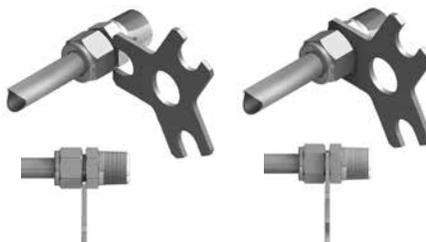
On initial installation, the Swagelok gap inspection gauge assures the installer or inspector that a fitting has been sufficiently tightened.
