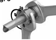
1. Insert the tube with preswaged ferrules into the fitting until the front ferrule seats against the fitting body; rotate the nut finger-tight (Fig. 1).
