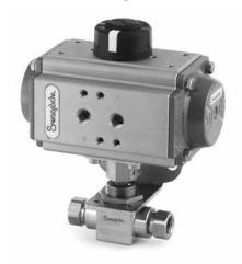
Swagelok ISO 5211-compliant rack and pinion pneumatic actuators are suitable for general applications. They are available in spring-return and doubleacting modes. On-off (2-way) valves require 90° actuation; switching (3-way) valves require 180° actuation.
