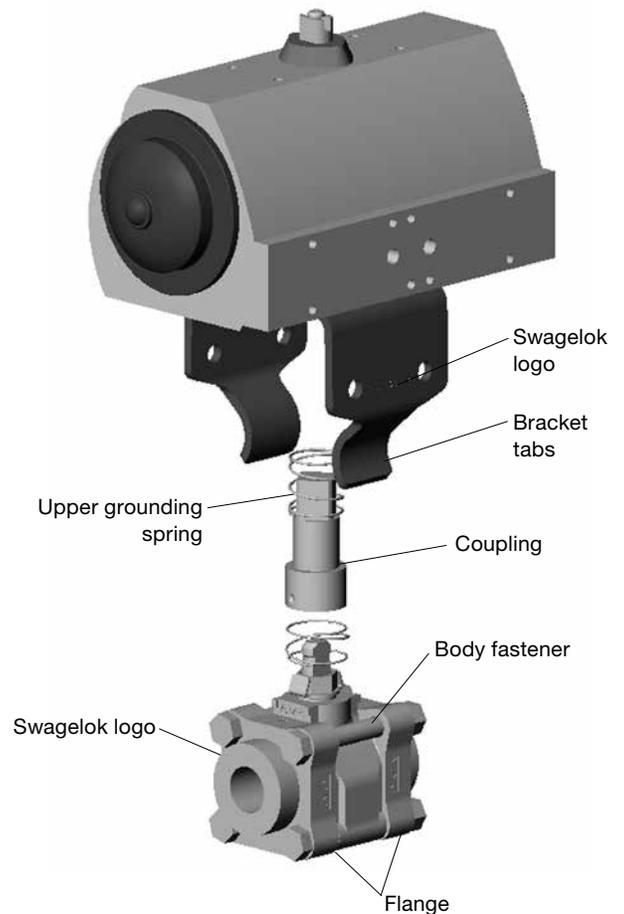
2. Place the **wall mount bracket** against the **actuator mounting bracket** on the side opposite the actuator bracket's **Swagelok logo**. If the wall mount bracket has a notch in the center, orient the notch towards the valve.
