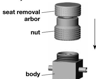
2. The **nut** should be fully tightened onto body with a **gap** showing between **nut** and **seat removal arbor**.
