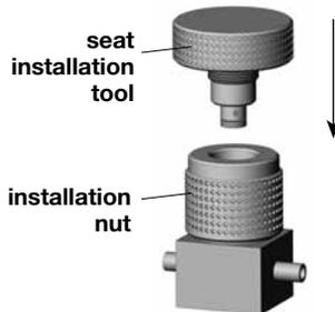
4. Loosen the **seat installation tool** several turns.
