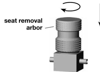
4. Remove **seat removal tool** from body by rotating **nut** counter-clockwise.
