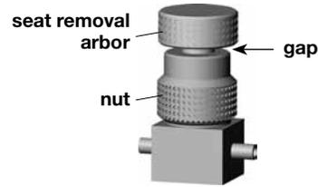
3. Apply slight downward pressure while turning the **seat removal arbor** clockwise. A drop in torque indicates the seat is removed from the body.
