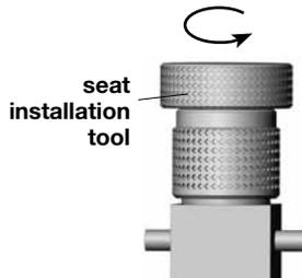
5. Remove the **seat installation tool** and **installation nut** from the body.
