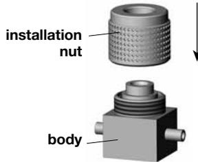
3. Thread the **seat installation tool** into the **installation nut** until contact is made with the seat. Continue turning the **seat installation tool** until the seat is firmly seated in the body. At this point, a significant rise in torque will be felt and the **seat installation tool** will be in close contact to the **installation nut**.
