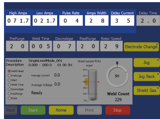
Fig. 63—Single Level Current-Control Group
