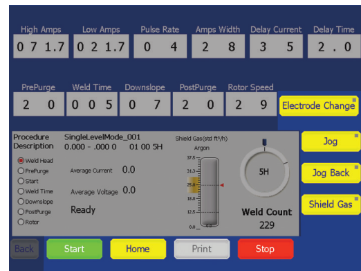
Fig. 65—Single Level Weld Process Buttons
