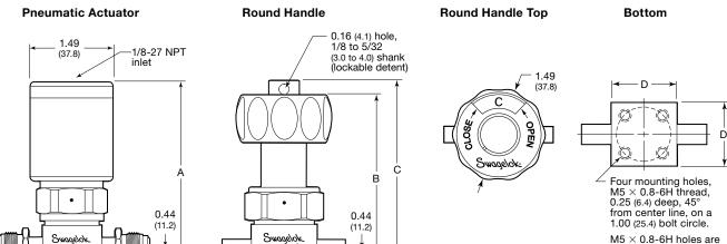
$M5 \times 0.8$ -6H holes are compatible with 10-32 mounting screws.
