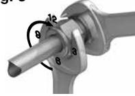
1. Insert the tube with preswaged ferrules into the fitting until the front ferrule seats against the fitting body; rotate the nut finger-tight (Fig. 1).
