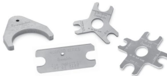
Swagelok gap inspection gauges assure the installer or inspector that the fitting has been sufficiently pulled up on initial installation, whether using a multihead hydraulic swaging unit (MHSU) or air-actuated hydraulic swaging unit (AHSU), or wrench tightening. All metal Swagelok tube fittings are gaugeable, with the exception of a few forged bodies in aluminum.
