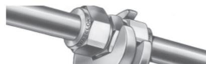
**⚠ Do not use the Swagelok gap inspection gauge with fittings that were assembled with a non-gaugeable preswaging tool.**
