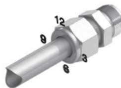
3. While holding the fitting body steady, tighten the nut one-half turn to the 12 o'clock position.
