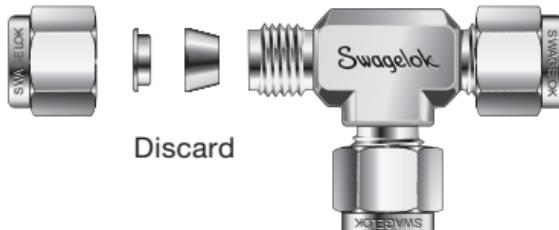
2. Slip the nut over the machined ferrule end of the port connector.
