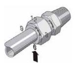
13. While holding the fitting body steady, tighten the nut one-half turn until the mark reaches the 12 o'clock position.
