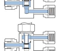
When there is no pressure to the actuator, the stem tip seals the lower port, allowing flow through the upper port.
